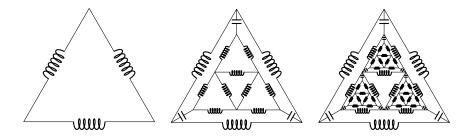
Capacitors  $Z_C = \frac{1}{i\omega C}$ , inductors  $Z_L = i\omega L$ .
